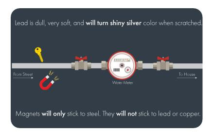
A service line is a portion of pipe that connects the water main to the building. To find out if you have copper, lead, galvanized steel, or plastic service on your property, you can perform a material verification test on the water service line where it connects to the water meter to determine of the service line.
